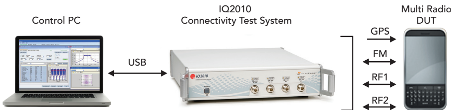
Figure 2: IQ2010 Test System—Testing Connectivity Functions of a Mobile Device
