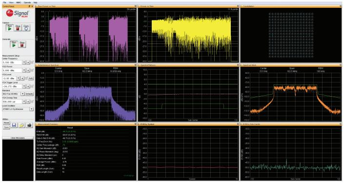
80 MHz 802.11ac test suite example: gated power vs. time, constellation, spectrum flatness/mask, EVM, Pilot EVM, Data & pilot EVM, TX freq. error, center freq. leakage, I/Q gain/phase/delay mismatch, peak/average power.
