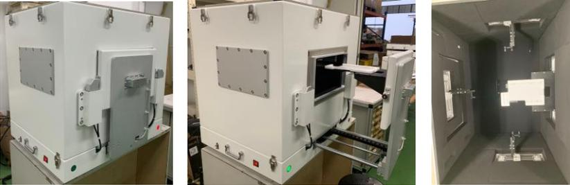
Chamber (DFF) without device positioner (or simple device positioner)
