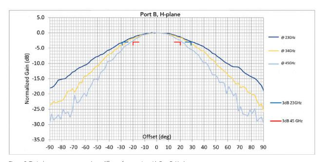
Figure 8: Typical antenna patterns at three different frequencies with Port B, H-plane
