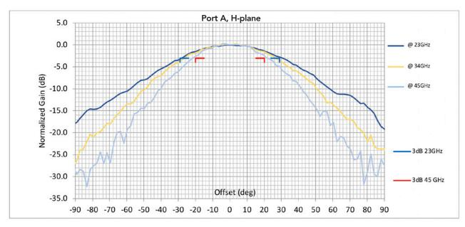
Figure 7: Typical antenna patterns at three different frequencies with Port A, H-plane
