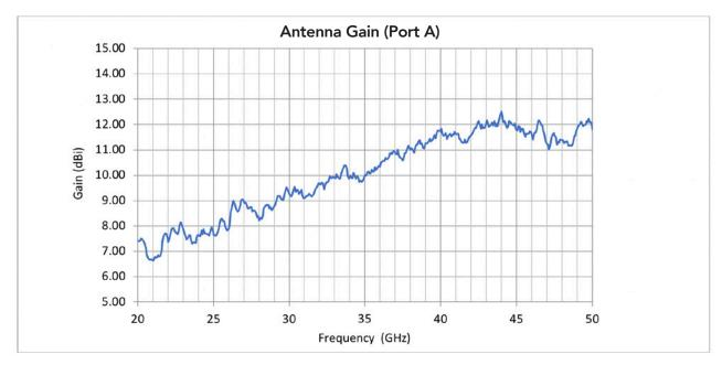
Figure 2: Antenna Gain, Port A
