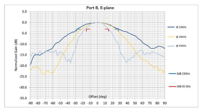
Figure 10: Typical antenna patterns at three different frequencies with Port B, E-plane
