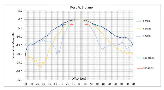
Figure 9: Typical antenna patterns at three different frequencies with Port A, E-plane
