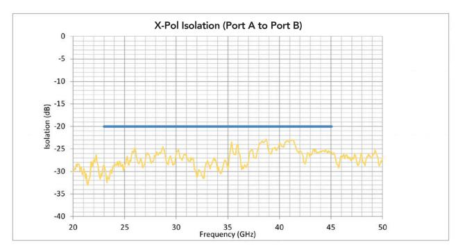
Figure 5: Cross Polarization Isolation Port A to Port B
