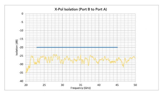
Figure 6: Cross Polarization Isolation Port B to Port A
