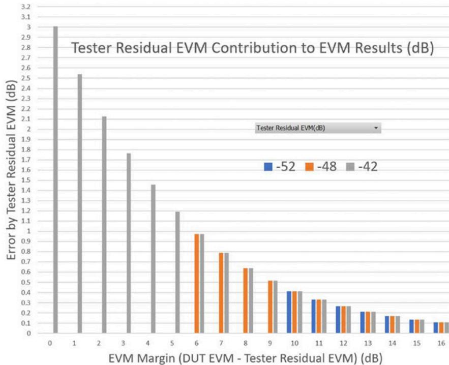
Figure 5: Measurement error contributed by tester's EVM floor
