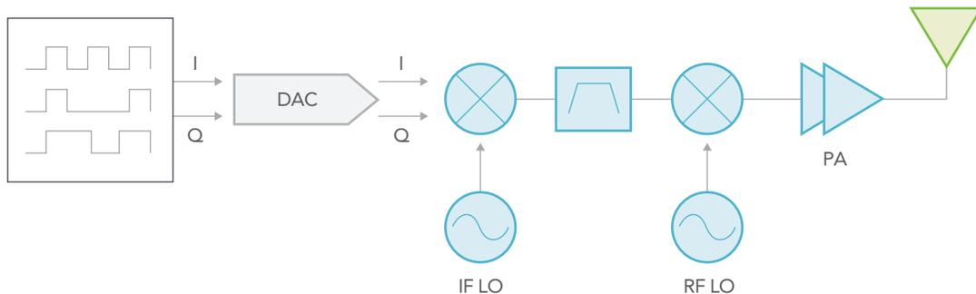
Figure 1: Simplified transmitter block diagram
