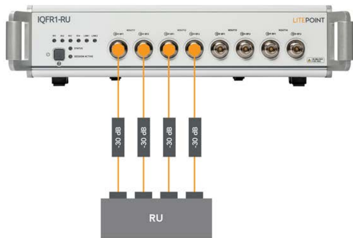
Figure 7 IQFR1-RU Wide Area Base Station Simple Setup with SC-PSD Aided
